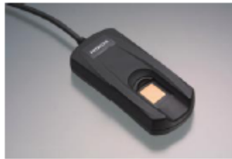
Fig. 4—Finger-vein Scanner. The finger-vein scanner detects the finger-vein pattern and sends it to the controller.
