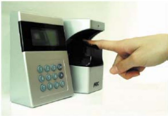
Fig. 4—Finger-vein Scanner. The finger-vein scanner detects the finger-vein pattern and sends it to the controller.
